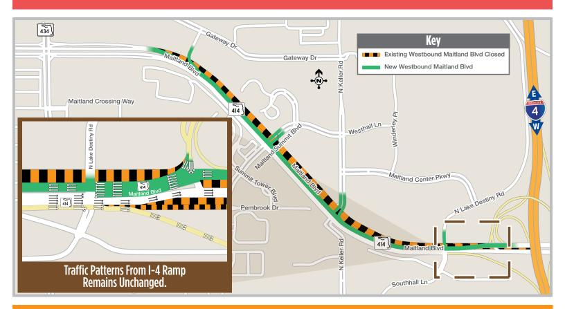
This long-term traffic pattern of approximately 1.25 miles in length will relocate the westbound lanes to new pavement south of the existing traffic lanes. The new traffic pattern is necessary for the reconstruction of Maitland Boulevard. Exact date of the ramp closure will be available on i4Ultimate.com/alertsmap.
