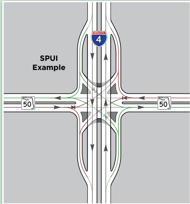
A single-point urban interchange (SPUI) is a type of interchange that is used to safely and efficiently move large traffic volumes through an intersection with limited amount of space. A SPUI allows opposing left turns to proceed simultaneously in one single intersection over or under the free-flowing road — the I-4 Ultimate project will have examples of both of these Colonial Drive will have a SPUI under I-4 and State Road 436 will have a SPUI above I-4.
